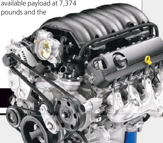
2014 GM ECOTEC3 6.2-LITER V-8 ENGINE
