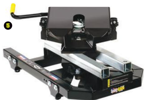
(1) Reese Sidewinder fifth-wheel pin box. Three WD systems with sway control: (2) Blue Ox Sway Pro, (3) Pro Series Friction Sway Control, (4) Reese Strait-Line. (5) PullRite SuperGlide sliding fifth-wheel hitch.
